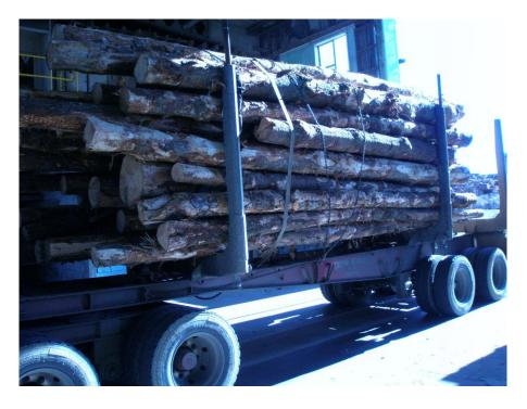
This load recently turned up at our Kinleith log yard. The investigation discovered that the driver noticed the log that wasn't between the two staunchions once he had MOVED AWAY from the loader operator, to the chain up area. The driver decided not to go back and get the load adjusted because the truck behind him had already started to be loaded, so put an extra chain and strap on instead.
