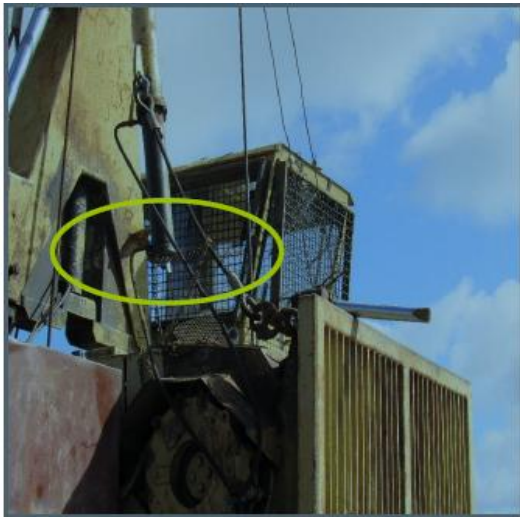
Figure 2. Close up of the hauler showing snapped spear
